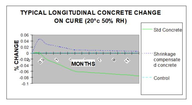
As you can see from the graph, you could expect a standard 5m x 5m grid design concrete floor to shrink up to 2mm around each grid perimeter (4mm total longitudinal shrinkage over 5 metres).
