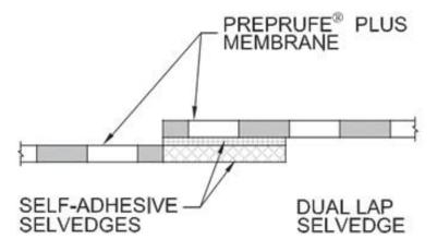
ASSEMBLY (PLAN OR SECTION VIEW)
