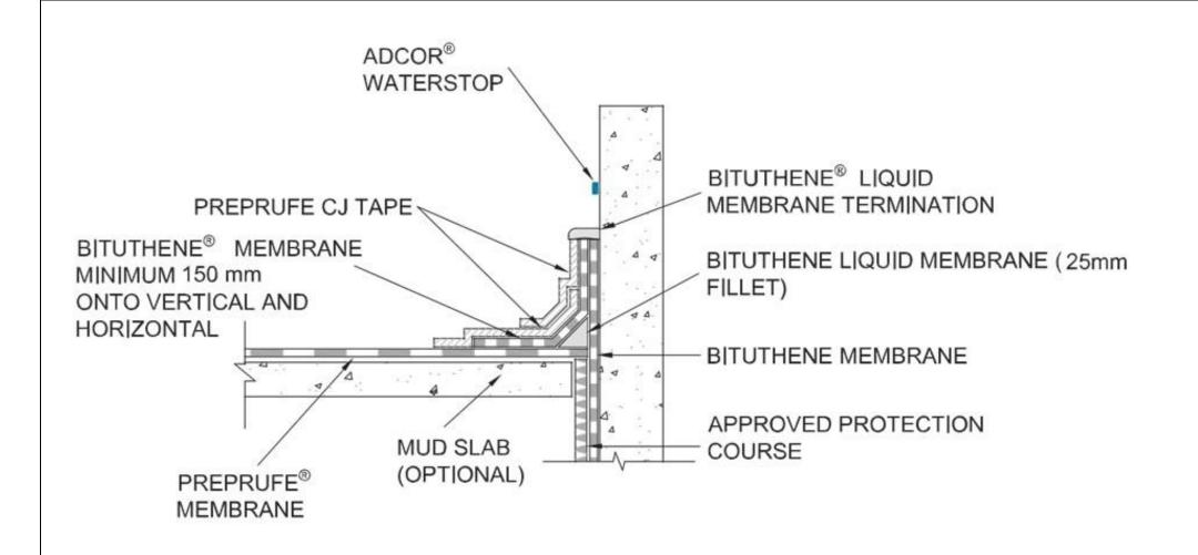
NOTES - IF A MUDSLAB IS NOT USED, THE SUBSTRATE TO ACCEPT THE BITUTHENE LIQUID MEMBRANE MUST BE GROUTED SOLID TO PROVIDE AN ACCEPTABLE SUBSTRATE FOR THE LIQUID MEMBRANE
