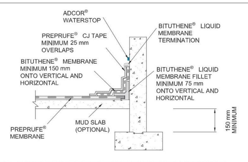
NOTES - IF A MUDSLAB IS NOT USED, THE SUBSTRATE TO ACCEPT THE BITUTHENE LIQUID MEMBRANE MUST BE GROUTED SOLID TO PROVIDE AN ACCEPTABLE SUBSTRATE FOR THE LIQUID MEMBRANE - INTENDED FOR PROJECTS WITH PERMANENT DEWATERING OR NON-HYDROSTATIC CONDITIONS
