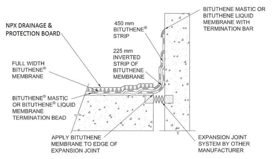
NOTES: - FOR JOINT WIDTHS UP TO 2 IN. (50 mm) WITH A MAXIMUM OF 1 IN. (25 mm) MOVEMENT. IF EXPECTED MOVEMENT IS LESS THAN 0.5 IN. (15 mm) A 6 in. (150 mm) INVERTED STRIP IS ACCEPTABLE - A WATERPROOF EXPANSION JOINT SYSTEM BY OTHERS MUST BE SELECTED FOR THE WIDTH AND EXPECTED
