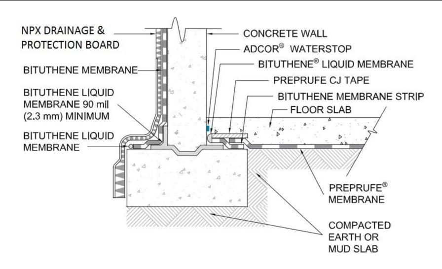
NOTES: -THE FOOTING KEYWAY SHOULD BE FORMED TO CREATE A REGULAR AND UNIFORM SHAPE ALLOWING PROPER DETAILING OF THE BITUTHENE LIQUID MEMBRANE.
