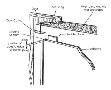
BioClad hygienic wall system 2.5mm thick is installed over most dry substrates, to quarry tile base/skirting (typical 100mm by 12mm thick) with similar floor tiles fixed with Nuplex NPU 2 Part Adhesive and double-sided tape sealed with silicone sealant.
